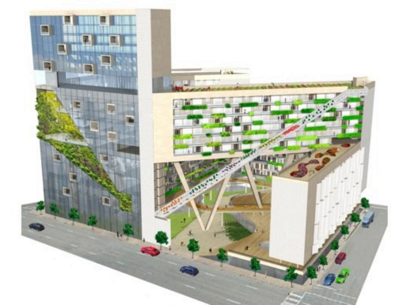
Re-used and e-invention of super cell structurel system that capable of securing 4 retired fuseleges. esult: plugged and played system was developed for the building construction. re-condition Fuselage stacking up on each other at its NO columns natural state. NO floor sleps Big cost saving Pre - Wire for Mechanical. Electrical. Mumbing. systems \_\_ \_Proposed Future
